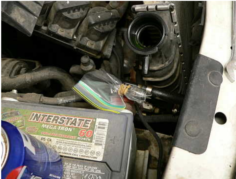
Figure 4 - A baggie rubber-banded over the trans lines helps control the mess.
